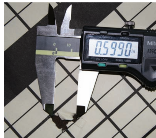
Digital calipers were used to measure the group size for the precision shooting test, using the extreme spread.
